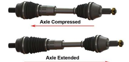
Axle shaft telescopes to provide
