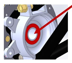
**STEP TWO:** Once you have the item elevated and the old axle is removed you need to get a measurement from the face of the differential to the inner face of the wheel hub.
