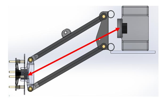
**STEP THREE:** Once you have taken the measurement you need as indicated by the RED line you have successfully measured that axle at full droop. You can then lower the vehicle back to the ground to take measurements for the compressed level.
