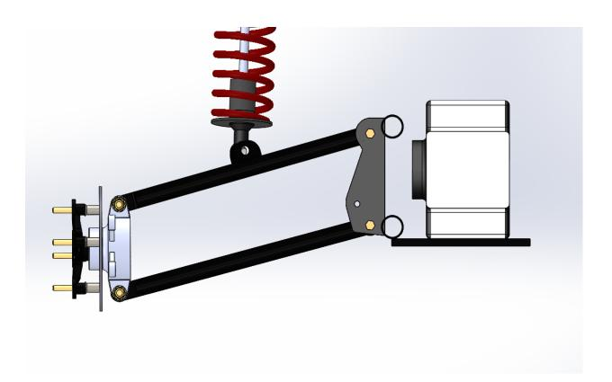
**STEP FOUR:** Once the vehicle is back on the ground you will need to take the same measurements. The reason being to get your compressed length. This is necessary to give your vehicle the best functionality at performance.
